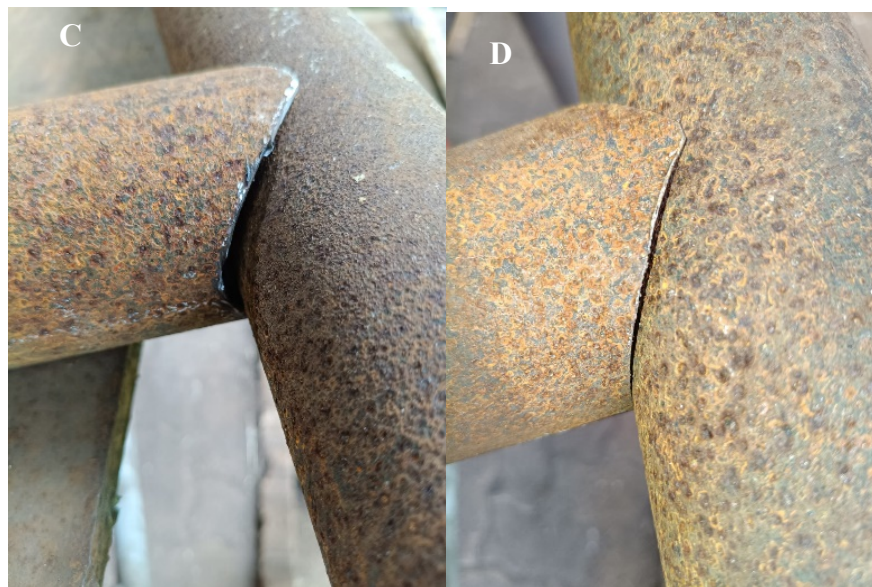
Figure 6. Pipe Connections: C. Manual D. Using a Pipe Notcher.
