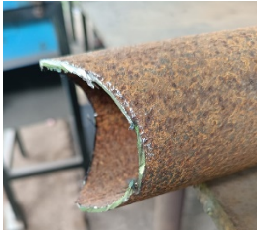
Figure 1. Observation Results: the manual method resulting the pattern is rougher
