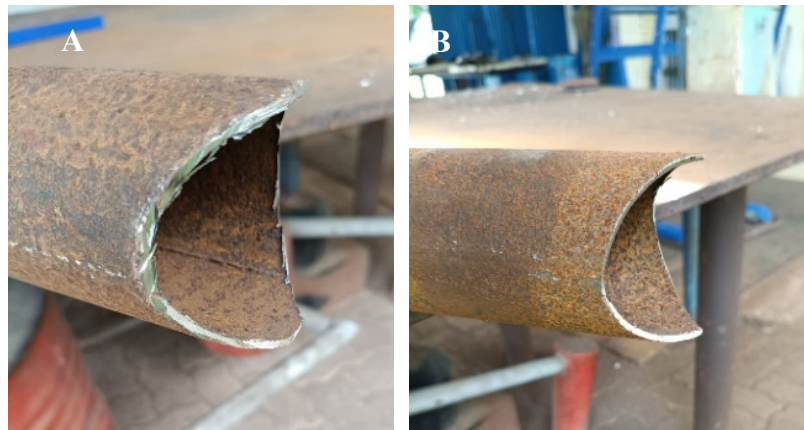
Figure 5. Results of notching on pipes: A. Manual B. Using a Pipe Notcher Tool
