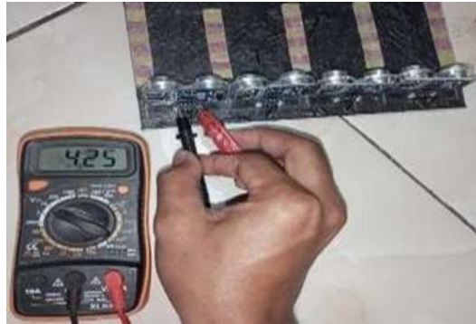
Figure 8. Ultrasonic voltage measurement of slot 1
